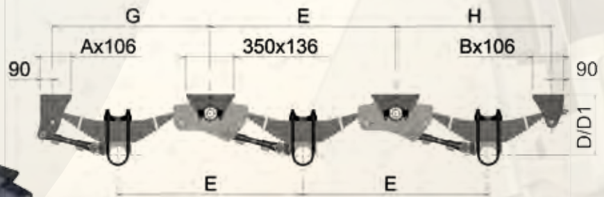
TRI AXLE SUSPENSION TYPE N WITH SPRING WIDTH 75 TRIDEM TYPE N A RESSORTS DE 75
