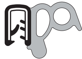
Edge protection and sealing profile Weight 0.31 kg/m.
