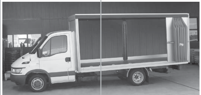
Illustration: fully assembled body kit showing the optional extras - curtains, centre pillar, and floor side planks.
