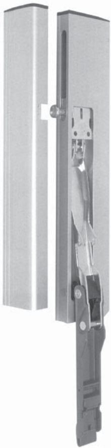
Illustration: When opening, the hand lever folds down completely and lies on the side board. The illustration shows a left hand assembly.
